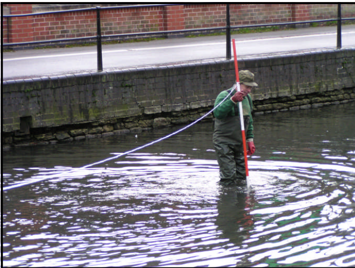
Dave Pullen checking the river bed levels for winding hole.
